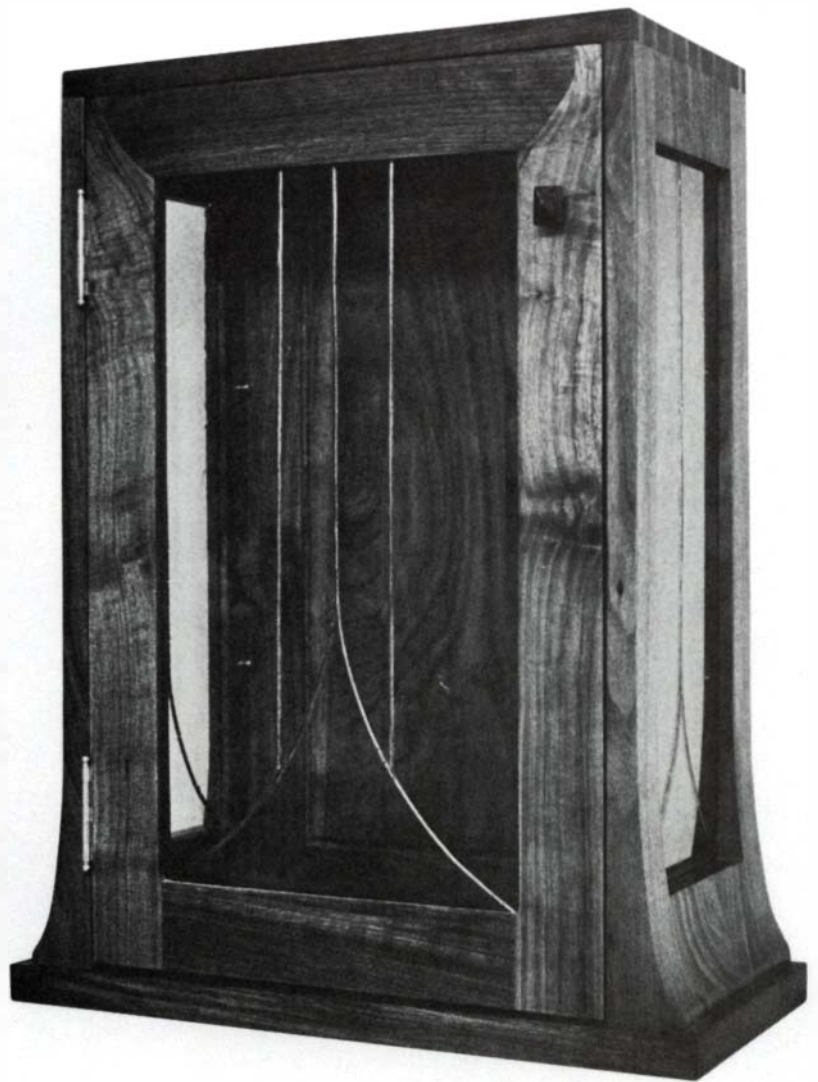
The door on this cabinet shows how contoured joinery can be used to advantage. The wood has been carefully selected so the grain conforms to the curvature of the joint, which repeats the gentle curve made by the bottom sides of the cabinet. The two bottom joints of the door frame have been cut square, complementing the upper corners of the case.
